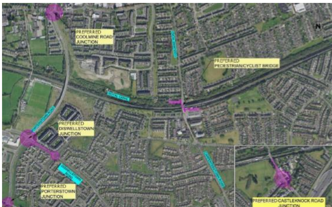
Figure 4-3 Coolmine level crossing replacement preferred option
